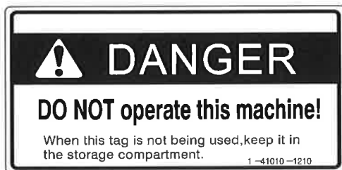
(19) Warning tag to prevent operation during maintenance (1-41010-1210)
