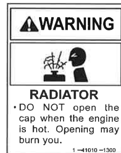
(12) Beware of high-temperature coolant (1-41010-1300)
