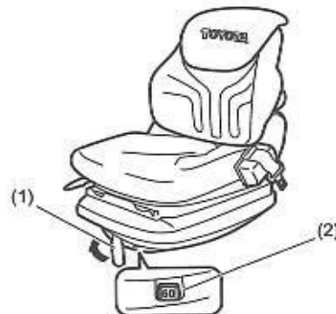
(1) Weight adjustment lever (2) Indicator
