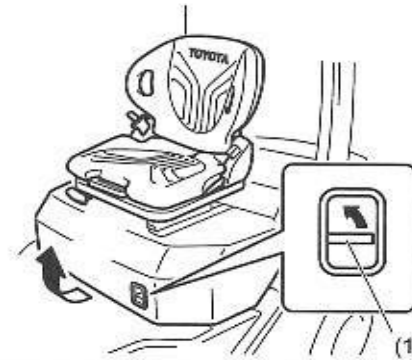
(1) Engine hood lock release lever
