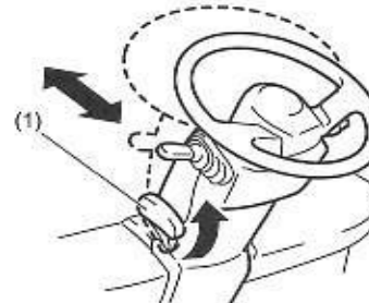
(1) Tilt steering adjusting lever
